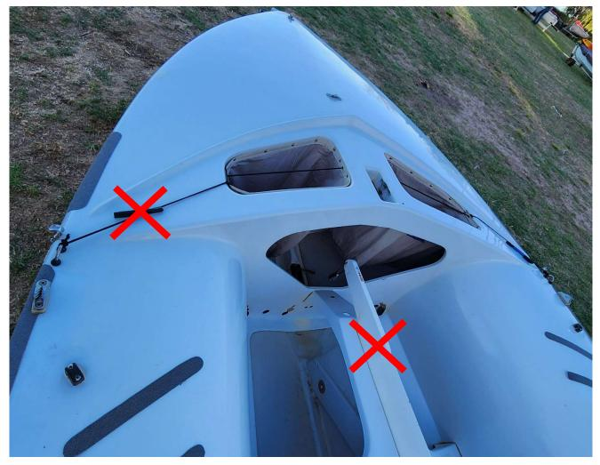
Centreboard has to be removed and also the Spinnaker halyard holders.
